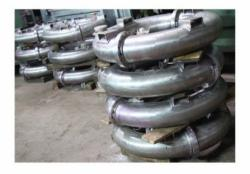
Pipe Bends, 3d Bends, 'U' Bends Range 1/4" X(6mm) to 24" X(600mm) Wall Thickness up to 50mm
